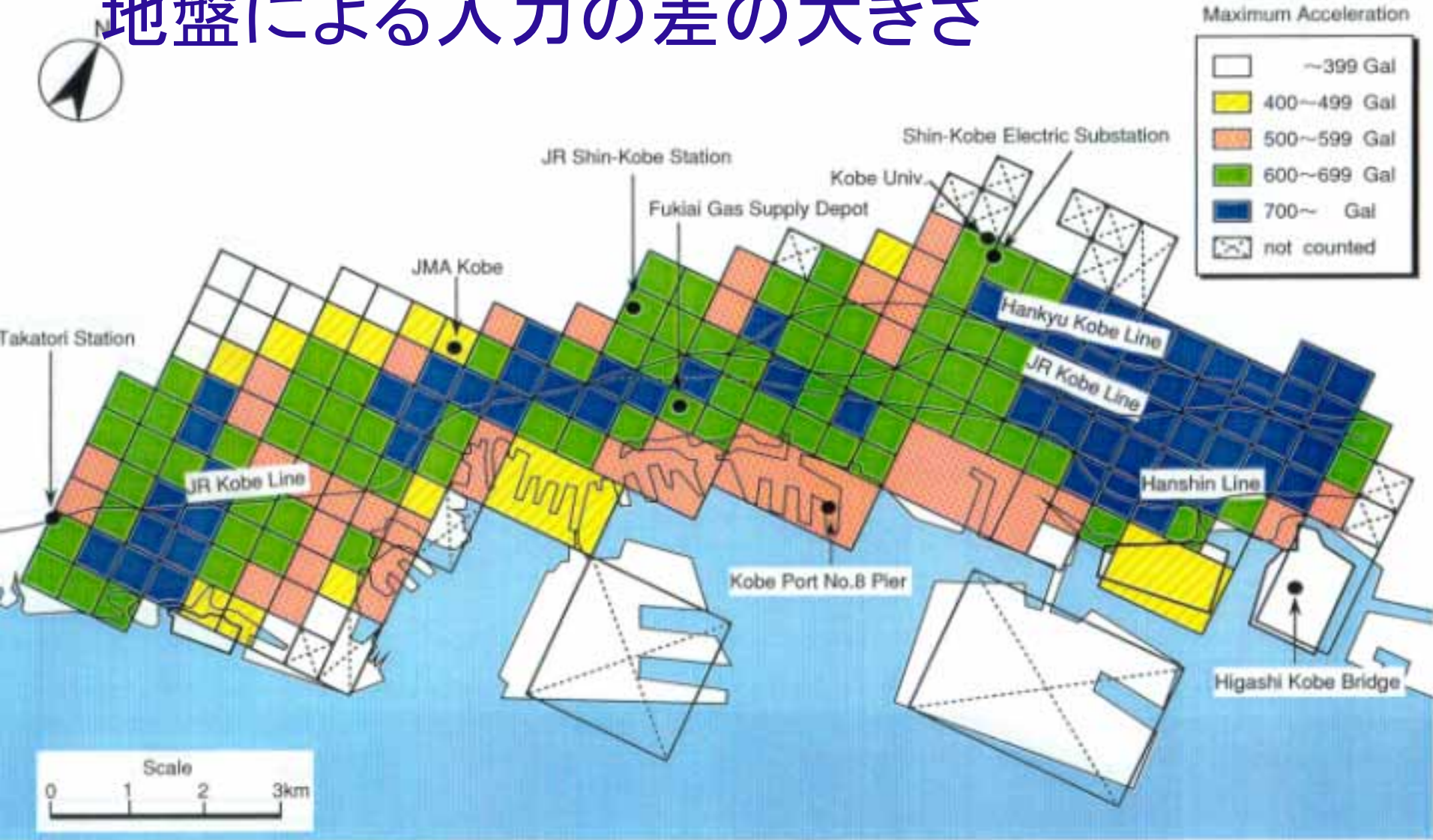
Fig.6 Distribution of maximum acceleration for macro-analysis based on Sato's results 12)
